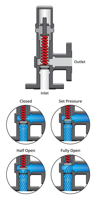
Guided piston relief valve in action: As pressure on the line increases, the spring-loaded piston opens the valve and diverts the flow to maintain the set pressure.
