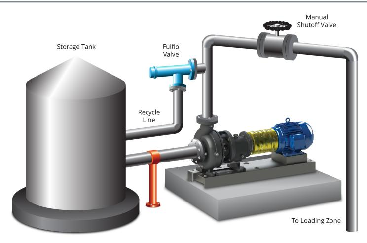
Solution: Guided piston relief valve maintains consistent line pressure and protects pump
