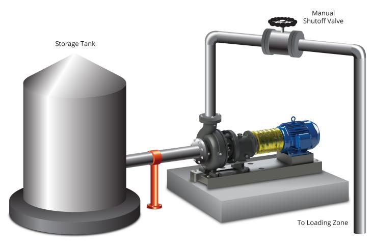
Problem: Manual shutoff valve puts pump at risk for overpressure
